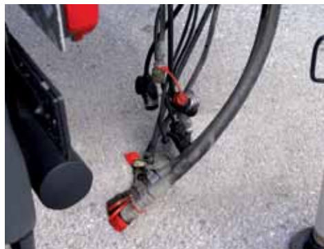
Disconnect hydraulic power supply
