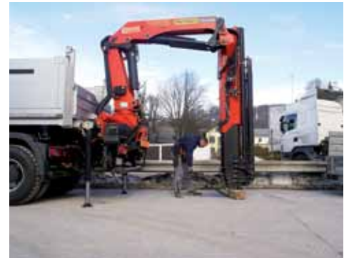
Stabilize over the tip of the crane boom
