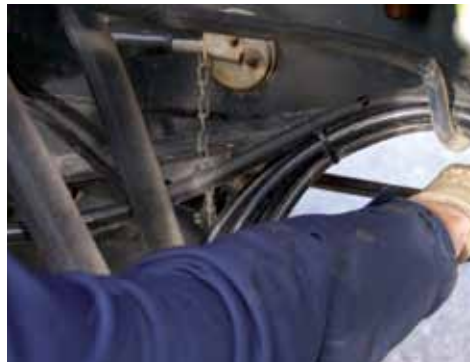
Release holding clip and clamping claw
